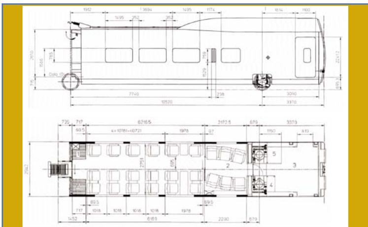
The total length of the train is about 200 m, and the average length of coaches is 13,14 m. That dimension will be taken as a reference for defining the geometry of the coach tested.
